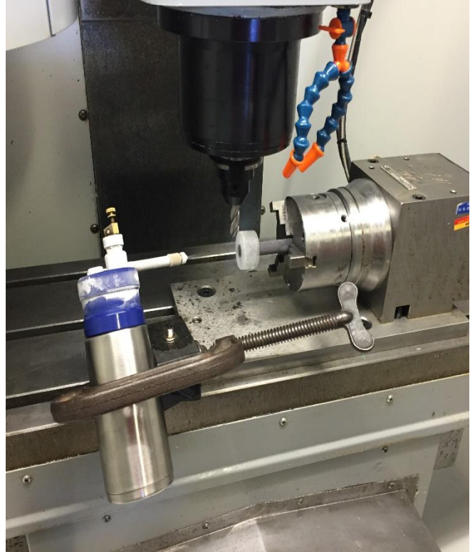
Figure 3.8 – Machining setup, coolant position along with ice infiltrated sample
